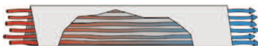
Traditional catalyst element – straight-line laminar flow: Most exhaust gas never contacts the catalyst.
