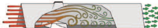
NEXT channel grooves create exhaust gas turbulence for more pollutant breakdown – and superior durability.
