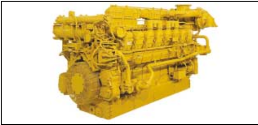
One of the Okemo Mountain Resort's primary engine-driven air compressors for snowmaking comprises a Caterpillar 3516B diesel similar to the unit pictured, driving an Ingersoll-Rand Centac 2ACII57D3 compressor. The Miratech SCR system reduced NO x by 85% on the engine without any operational problems.
